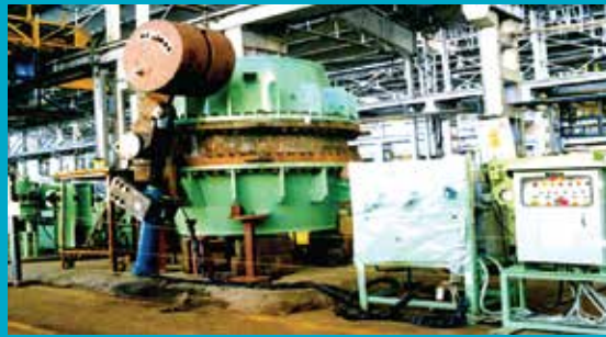
Proof of design tests on 2400mm pump discharge butterfly valve was conducted as per AWWA C 504. The valve was successfully tested and approved by NTPC.
