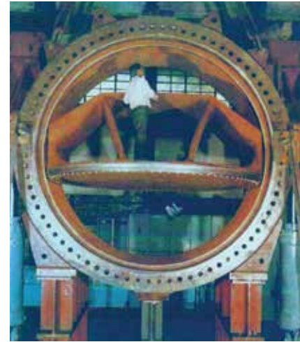
3700mm(30bar) penstock protection butterfly valve supplied to Bhira Hydro Power plant of TATA Power
