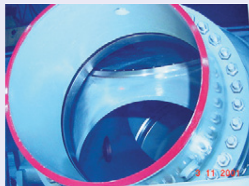
Details of the movable seat ring on the body
